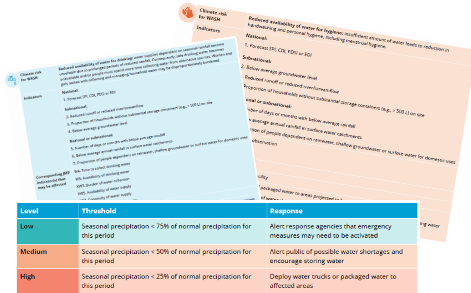
Figure 1. Examples of thresholds for an indicator of the risk of reduced precipitation creating shortfalls in local water supplies
